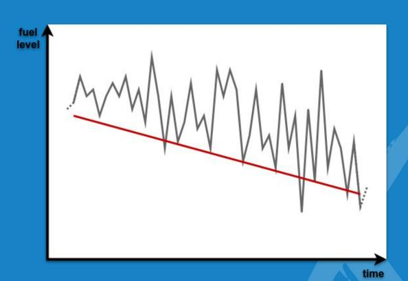
We use median filtration in Wialon. You can set it up with a help of filtration level. The bigger level you set – the wider sliding window is used to calculate smoothed value in the middle.
