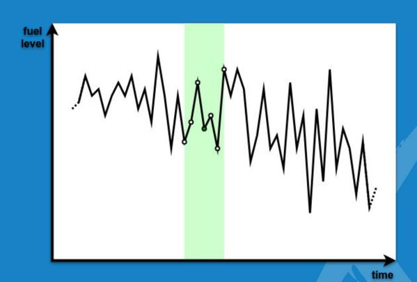
We use median filtration in Wialon. You can set it up with a help of filtration level. The bigger level you set – the wider sliding window is used to calculate smoothed value in the middle.
