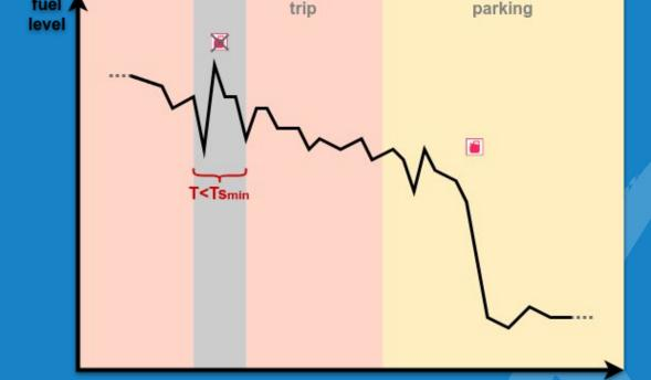
Usually fillings detection is done for the whole FLS data, but the following option can exclude movement.
