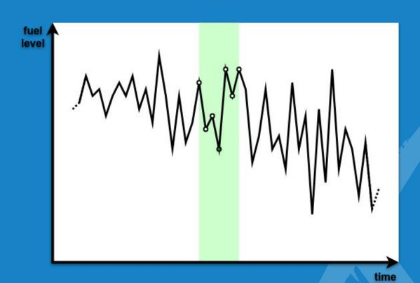
Even after filtration there will be some fluctuations left. So we need to separate these fluctuations from fillings and thefts with a help of rough filter – minimum fuel filling and theft volume (VFmin & VTmin).
