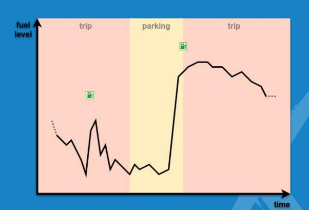
Usually fillings detection is done for the whole FLS data, but the following option can exclude movement.
